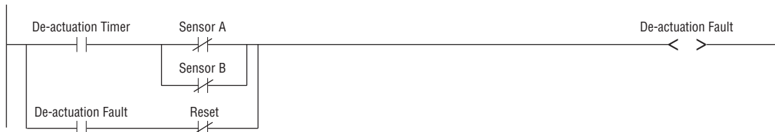
De-actuation Fault Monitoring Ladder Logic Example
