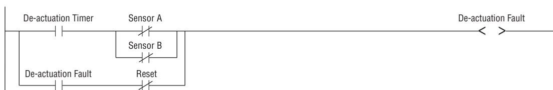
De-actuation Fault Monitoring Ladder Logic Example
