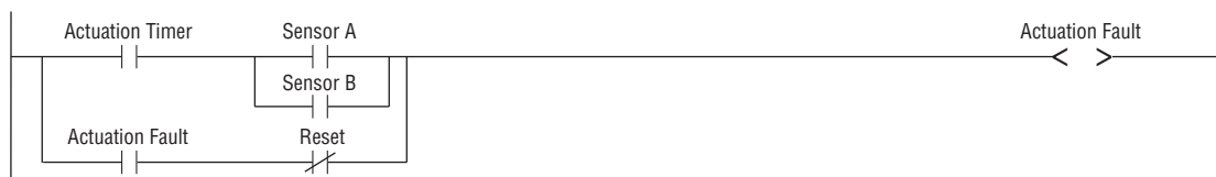
Actuation Fault Monitoring Ladder Logic Example
