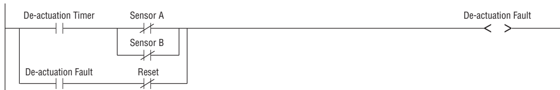
De-actuation Fault Monitoring Ladder Logic Example
